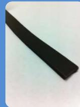
Foam tape is used to create channel in spray made bag to allow for use of tacky tape in autoclave applications.
