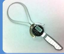
Calipers used to measure minimum bag thickness of 0.125in.
